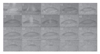
Figure 6. Sequence of ceramic ink drop impact on previous film of ceramic ink on ceramic substrate under gravity from burette nozzle. nozzle dia=2mm, stand-off distance from substrate=25mm (ethyl alcohol, 13 vol % of alumina and 1 vol % of dispersant).
