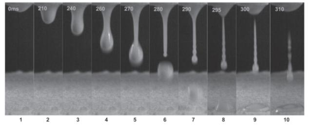
Figure 3. Sequence of formation of ceramic ink drop under gravity from burette nozzle. nozzle dia=2 mm, stand-off distance from substrate=25 mm, interframe time=0.005 s (ethyl alcohol, 13 vol % of alumina and 1 vol % of dispersant).
