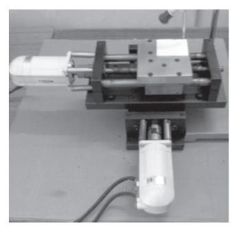
Figure 2. X-Y table for position control.
