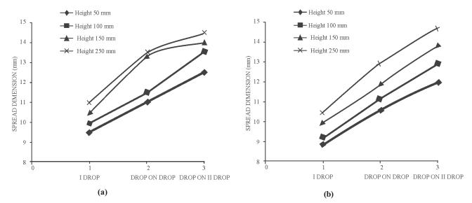
Figure 9. Variation of drop spread when drop impinges a previous drop on substrate for different stand-off distances: (a) ethyl alcohol, 13 vol % of alumina and 1 vol % of dispersant (b) ethyl alcohol, 12.5 vol % of zirconia and 1 vol % of dispersant.
