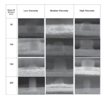
Figure 5. First drop impact on substrate under gravity, for different apparent viscosities of alumina-based ink and for different stand-off distances from substrate.
