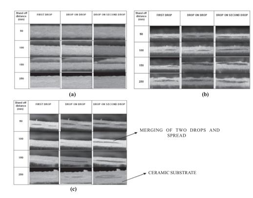
Figure 11. Convergence of two ceramic ink drops on substrate under gravity, for varying apparent viscosities of ink and stand-off distances: (a) ink with low viscosity, (b) ink with medium viscosity, and (c) ink with high viscosity.
