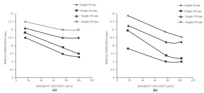
Figure 8. Variation of drop spread on substrate for different apparent viscosities of ceramic ink at different stand-off distances: (a) alumina-based ink, and (b) zirconia-based ink.
