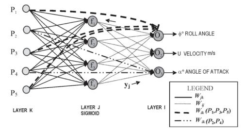
Figure 2. 5-4-3 neural network architecture model.
