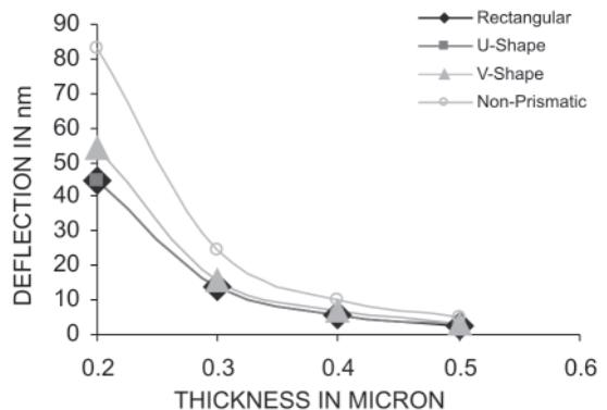
Figure 12. Deflection versus thickness of different shaped microcantilevers (shapes a to d).
