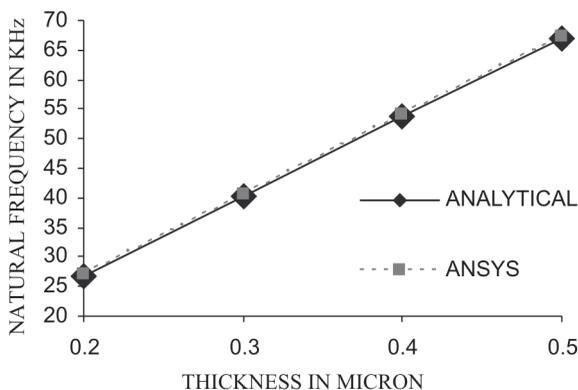
Figure 15. Natural frequency of rectangular cantilever calculated analytically and by ANSYS.
