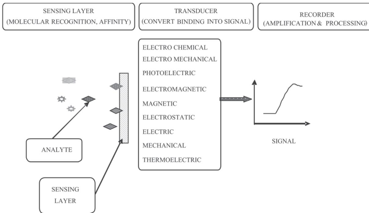
Figure 1. Schematic of general sensor design.
