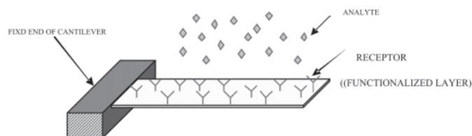
Figure 2. Microcantilever-based biosensor.
