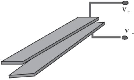
Figure 7. Capacitive method.
