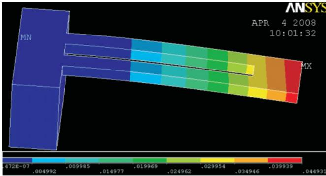
Figure 14. ANSYS output for the deflection of U-shaped microcantilever.
