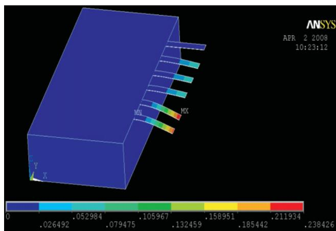
Figure 16. Deflection in microcantilever array.
