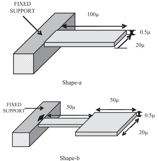
Figure 9. Two types of microcantilever geometries: (a) simple uniform beam fixed at one end and free at the other end, and (b) beam with narrow fixed-end and wide free-end.
