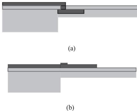
Figure 8. Piezoresistive method; cantilever cross-sections: (a) resistor on the bulk material and (b) resistor on a thin film.
