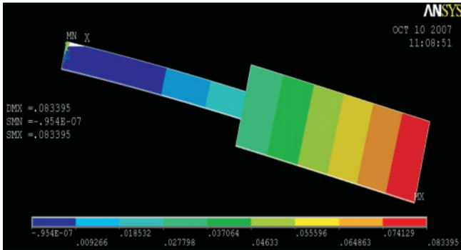
Figure 13. ANSYS output for deflection of microcantilever of shape-b.
