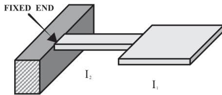
Figure 4. Cantilever with non-uniform area.
