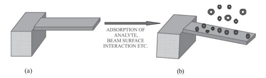
Figure 3. (a) Stress-free cantilever and (b) bending of the cantilever due to the generated surface stress by interaction with analyte.
