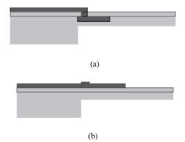
Figure 8. Piezoresistive method; cantilever cross-sections: (a) resistor on the bulk material and (b) resistor on a thin film.
