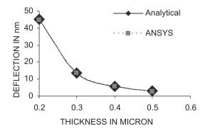
Figure 11. Deflection versus thickness calculated using analytical and FEM for rectangular shaped cantilever.
