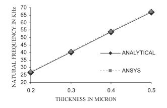
Figure 15. Natural frequency of rectangular cantilever calculated analytically and by ANSYS.
