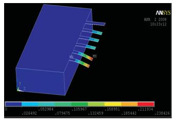
Figure 16. Deflection in microcantilever array.
