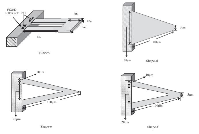
Figure 10. Structured cantilevers with U-shape and V-shape.
