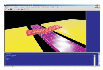
Figure 2. Screen shot of CPW switch showing the pull-in effect.
