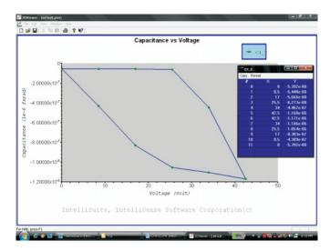
Figure 4. Capacitance vs voltage characteristics of the switch during pull-down and release.
