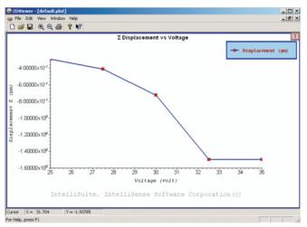
Figure 3. Reduction in gap height as a function of the applied voltage.
