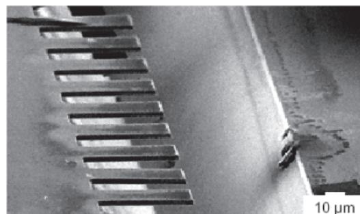
Figure 13. Micrograph of a beam array made by micro-machining<sup>47</sup>.
