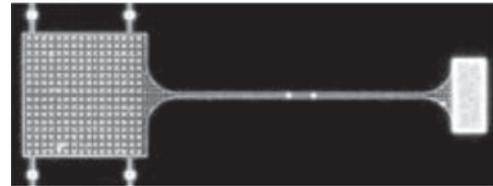
Figure 4. Polysilicon tensile specimen-3.5  $\mu\text{m}$  thick, 50  $\mu\text{m}$  wide, and 2 mm long<sup>36</sup>.
