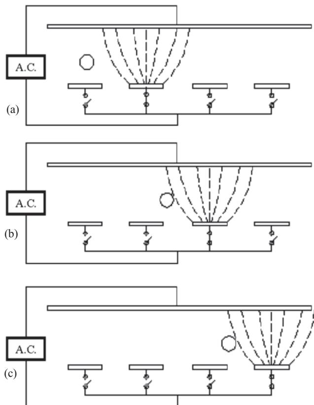
Figure 15. Schematic for moving electrophoresis.
