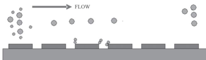
Figure 7. Flow separation by planar electrodes.
