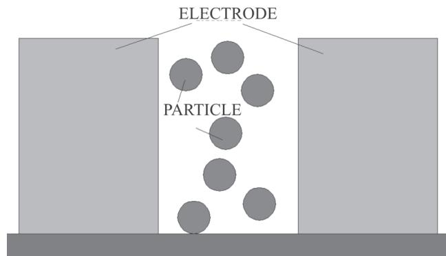
**Figure 11. DEP device with 3-D electrodes.**
