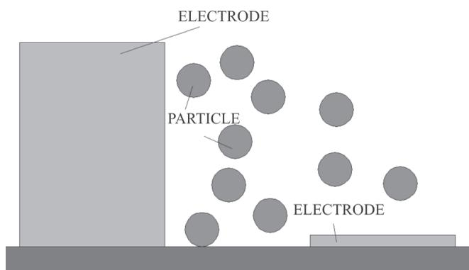
**Figure 13. DEP device with asymmetric electrodes.**
