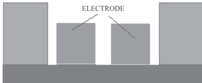
**Figure 10. DEP device with extruded electrodes.**
