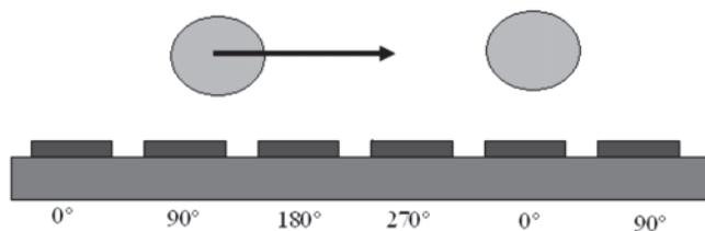
Figure 3. A schematic of travelling wave dielectrophoresis.
