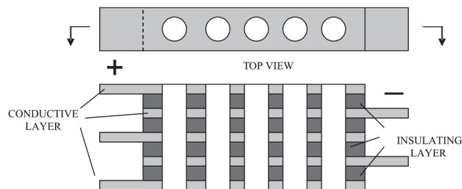
**Figure 14. 3-D composite DEP device with alternating conductive and insulating layer.**
