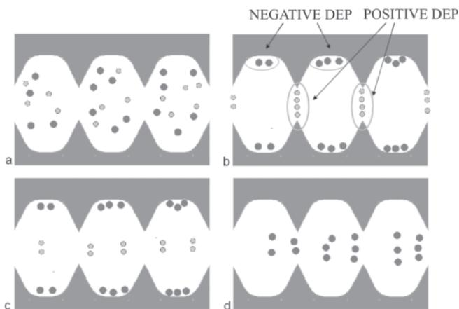
**Figure 12. Sequential field flow separation using DEP device with 3-D electrodes.**
