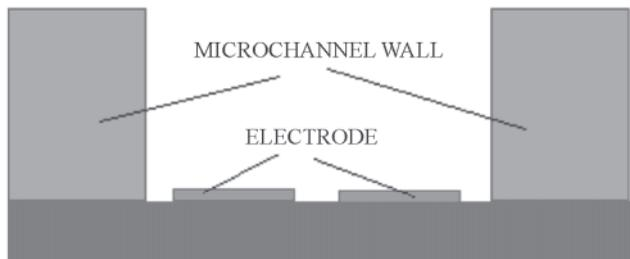
Figure 6. DEP devices with planar electrodes.
