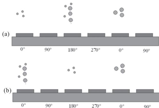
Figure 4. Separation using travelling-wave dielectrophoresis.
