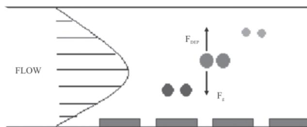
Figure 8. Field flow fractionation caused by flow speed profile of fluid.
