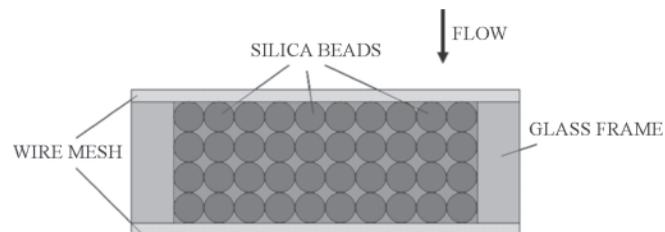
Figure 5. A schematic of 3-D DEP filter using silica beads.
