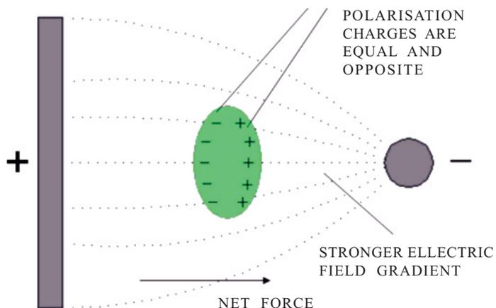
Figure 1. Principle of dielectrophoresis.
