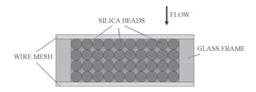
Figure 5. A schematic of 3-D DEP filter using silica beads.
