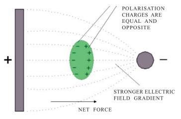
Figure 1. Principle of dielectrophoresis.
