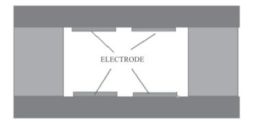
Figure 9. DEP device with two layers of electrode arrays.
