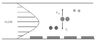
Figure 8. Field flow fractionation caused by flow speed profile of fluid.
