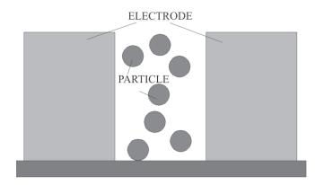
Figure 11. DEP device with 3-D electrodes.
