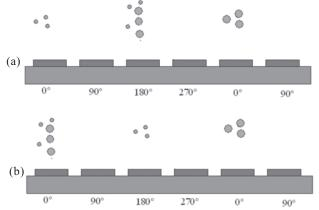
Figure 4. Separation using travelling-wave dielectrophoresis.
