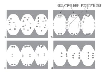
Figure 12. Sequential field flow separation using DEP device with 3-D electrodes.
