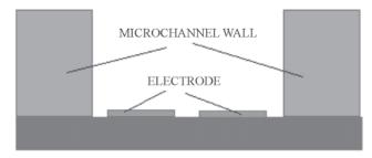
Figure 6. DEP devices with planar electrodes.
