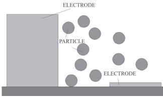
Figure 13. DEP device with asymmetric electrodes.
