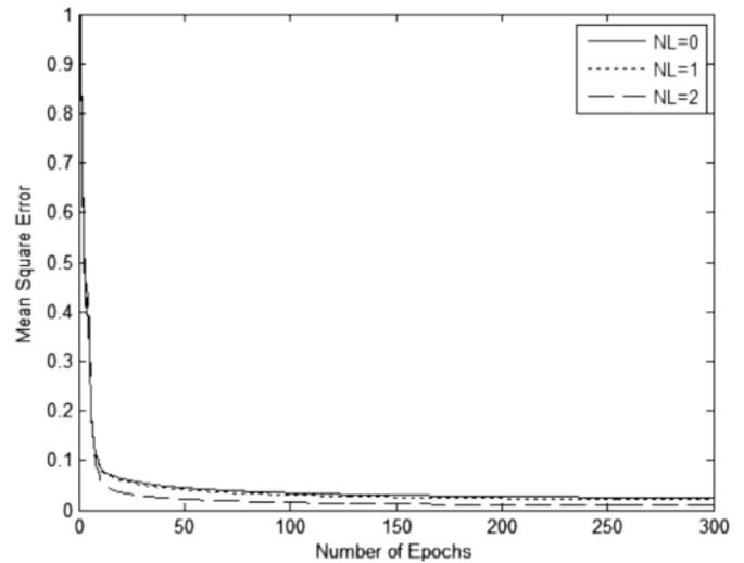
Figure 4. Convergence characteristic of the equalisers for the three channel models at SNR=16 dB.
