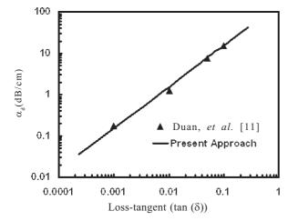
Figure 2. Variation of dielectric attenuation constant against loss-tangent ( $tan(\delta)$ ) of discrete dielectric support rod as computed using the present analysis and compared to those published in the literature [11] at 10 GHz.
