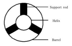
Figure 1. Schematic of a typical helix slow-wave structure.
