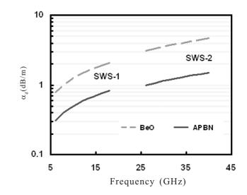
Figure 3. Variation of dielectric attenuation constant versus frequency for a C-Ku band (SWS-1) and a Ka band (SWS-2) slow-wave structures computed for the dielectric properties at 25 °C.
