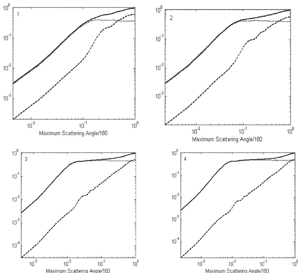
Figure 2. Beam efficiencies  $\eta_b$  (solid line) and  $\eta_{b0}$  (dashed line) and their difference (dotted line) of a dielectric sphere versus  $\theta_{lim}$  for refractive index  $m=0.603+6.37i$ ; size parameter: 1: $x=5$ , 2: $x=10$ , 3: $x=50$ , 4: $x=100$ .
