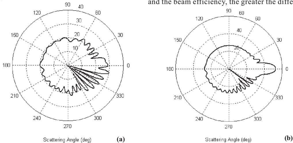
Figure 1. Angular scattering diagram in logarithmic (dB) scale (a) without and (b) with diffraction peak for a copper sphere,  $S_1$  upper semicircle,  $S_2$  lower semicircle.
