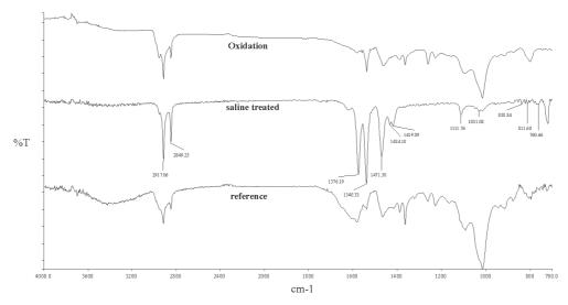
Figure 8. FTIR spectral changes for bromo-butyl rubber after 12-day environmental exposure.
