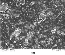
Figure 9. SEM images of: (a) reference and (b) temperature (120°C) -exposed for 36 h sample of bromo-butyl rubber.
