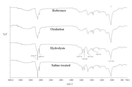
Figure 7. FTIR spectral changes for bromo-butyl after 4-day environmental exposure.
