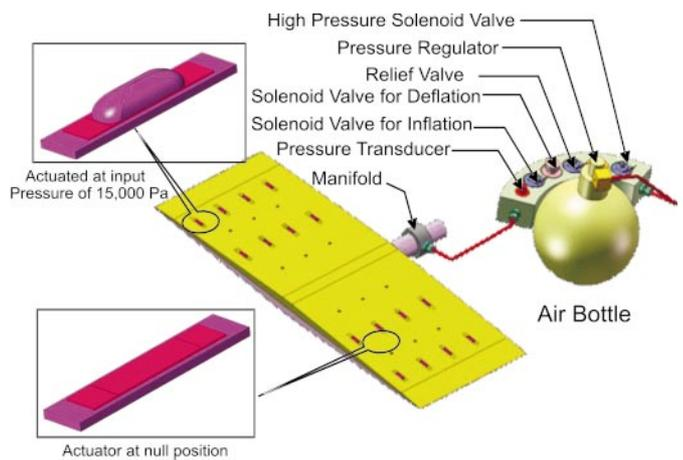
Figure 15. Details of pneumatic system and manifold.
