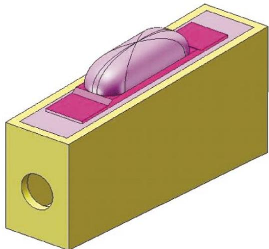
**Figure 3. Microballoon actuator with bigger height packaging.**
