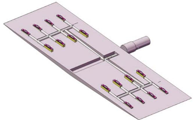
Figure 14. Embedded microballoon actuators with pneumatic tubes/pipes.
