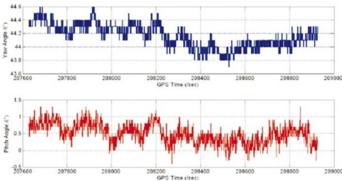
Figure 5. Single-baseline SD attitude results of static experiments.
