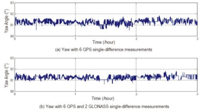
Figure 7. Yaw angle comparison between 6 GPSs and 8 GGs.
