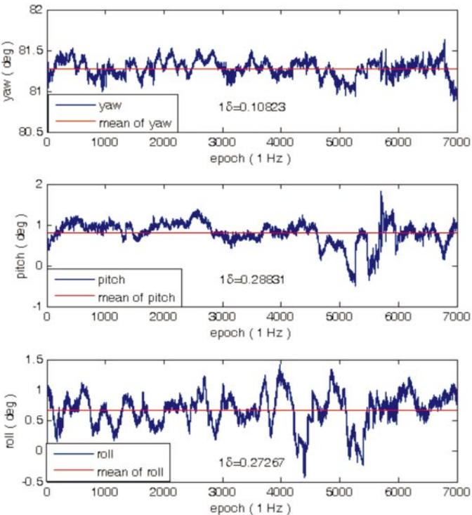
Figure 6. Double-baseline DD attitude results of static experiments.
