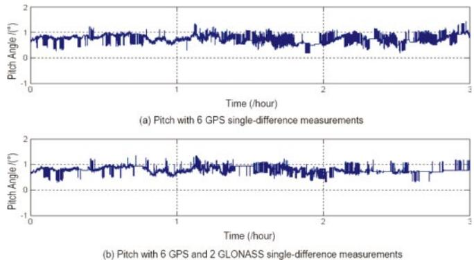
Figure 8. Pitch angle comparison between 6 GPSs and 8 GGs.
