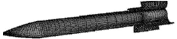
Figure 3. Meshing of body surface of standard TTCP projectile.
