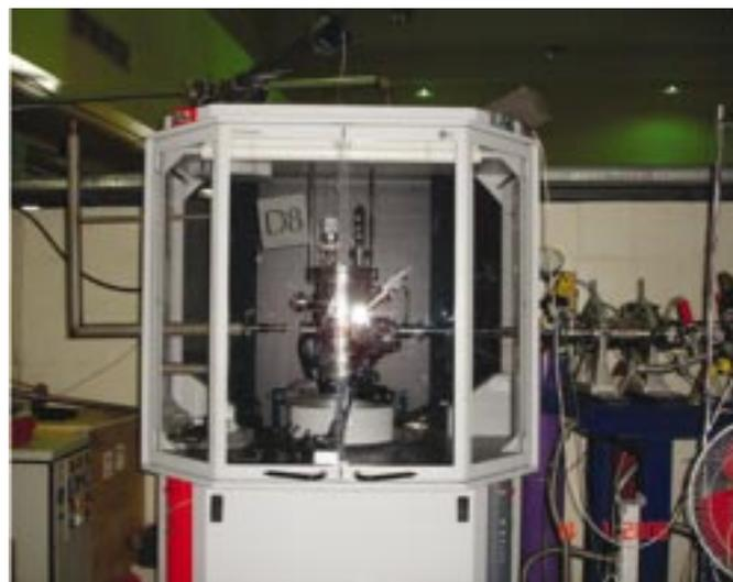
**Figure 9.** A view of *in-situ* X-ray diffractometer in the beam line. The chamber has a port to connect to the accelerator beam line. The chamber also has two Kapton (polyimide) windows for the entry and exit of the incident and diffracted X-rays respectively.
