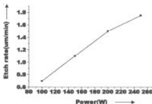
Figure 3. Etch rate variation with power. (Pressure = 100 mTorr,  $\text{CCl}_4 = 7 \text{ sccm}$ ,  $\text{CCl}_2\text{F}_2 = 35 \text{ sccm}$ , Time = 60 min).
