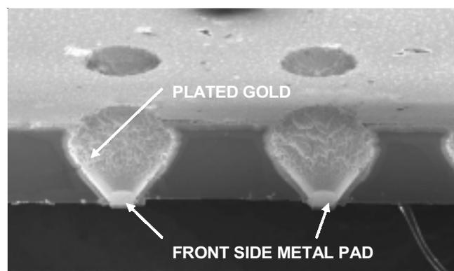
**Figure 8. SEM cross-section of 200  $\mu\text{m}$  deep plated via hole with good metal step coverage.**
