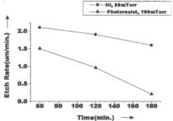
Figure 5. Etch rate variation with time. (power = 200 W,  $\text{CCl}_4/\text{CCl}_2\text{F}_2$  ratio = 1/5).
