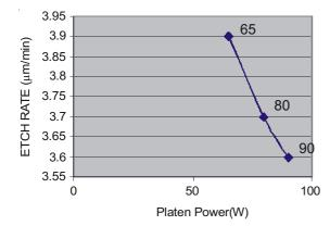
Figure 12. Etch rate as a function of platen power. (coil power = 950 W, pressure = 30 mTorr, etch time = 45 min)
