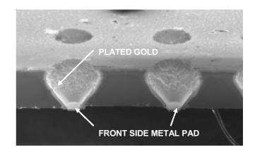
Figure 8. SEM cross-section of 200  $\mu$ m deep plated via hole with good metal step coverage.
