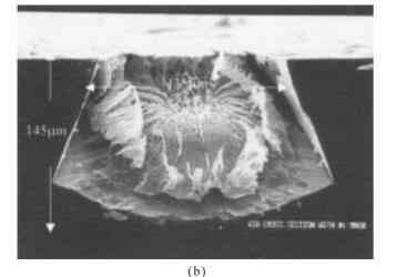
Figure 4. SEM via cross sections: (a) with photoresist mask, (b) with Ni mask.
