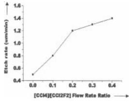
Figure 1. Etch rate variation with  $CCl_4$  to  $CCl_2F_2$  flow rate ratio. (Power = 200 W, Pressure = 100 mTorr).
