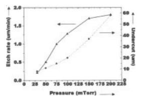
Figure 2. Etch rate variation and undercut obtained with pressure. (Power = 200 W,  $CCl_4 = 7$  sccm,  $CCl_2F_2 = 35$  sccm).
