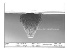
Figure 11. SEM cross-section of via-hole etched with 4.4 μm/min etch rate. (Coil power = 950 W, platen power = 80 W, etch time = 45 min)
