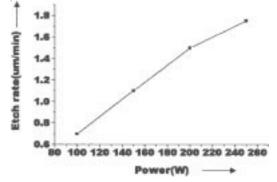
Figure 3. Etch rate variation with power. (Pressure = 100 mTorr,  $CCl_4 = 7 \text{ sccm}$ ,  $CCl_2F_2 = 35 \text{ sccm}$ , Time = 60 min).
