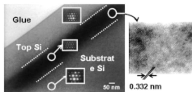
**Figure 2.** Bright field XTEM micrographs obtained from an as-implanted sample, which was further irradiated with 100 MeV O<sup>8+</sup> ions to the fluence of  $1 \times 10^{14}$  cm<sup>-2</sup> at 100 °C. The TEM image shows the top Si, the implanted layer, and the substrate Si. The dotted lines are a visual guide to demarcate the interfaces. The SAD patterns obtained from the three marked regions are also shown on the respective layers.
