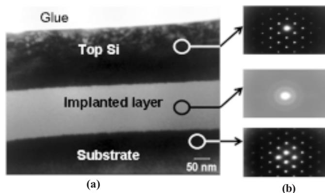
**Figure 1.** Bright field XTEM micrographs obtained from an as-implanted (100 keV N<sup>+</sup> ions) sample: (a) low magnification image showing the three distinct regions, and (b) SAD patterns ([110] zone axis of Si) obtained from the three marked regions in (a).
