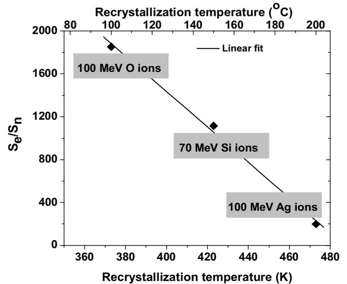
Figure 3. Variation in the recrystallisation temperature of the buried silicon nitride layer and the  $S_e/S_n$  ratio of different ions.
