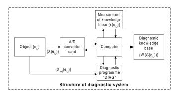
Figure 9. Scheme of diagnostic system with measurement module.
