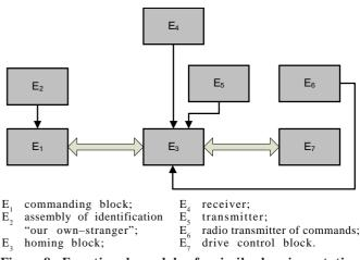
Figure 8. Functional model of missile homing station (NEWA SC).
