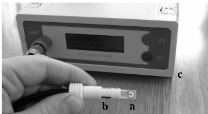
**Figure 2.** Photograph of used device. Screen printed sensor *a* with three electrodes is partially inserted into holder *b*. Output signal is measured using an amperometric potentiostat Bioanalyzer *c*.
