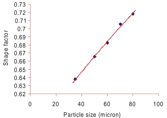
Figure 7. Effect of particle size of ground AP (APEP) on shape factor.
