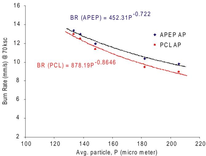
**Figure 2. Effect of particle size of AP on Burn rate of propellant compositions.**
