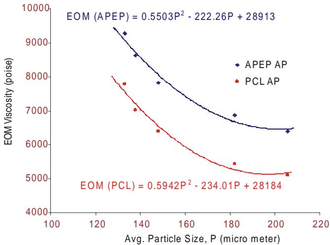
**Figure 1. Effect of particle size of AP on viscosity of propellant slurry.**
