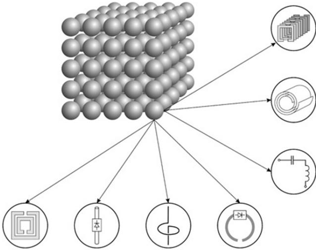
**Figure 1. Illustration of metamaterial concept in terms of conventional materials<sup>3</sup>.**
