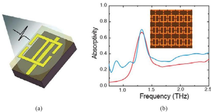
Figure 7. Metamaterial based absorbers for terahertz frequency region<sup>13</sup>.
