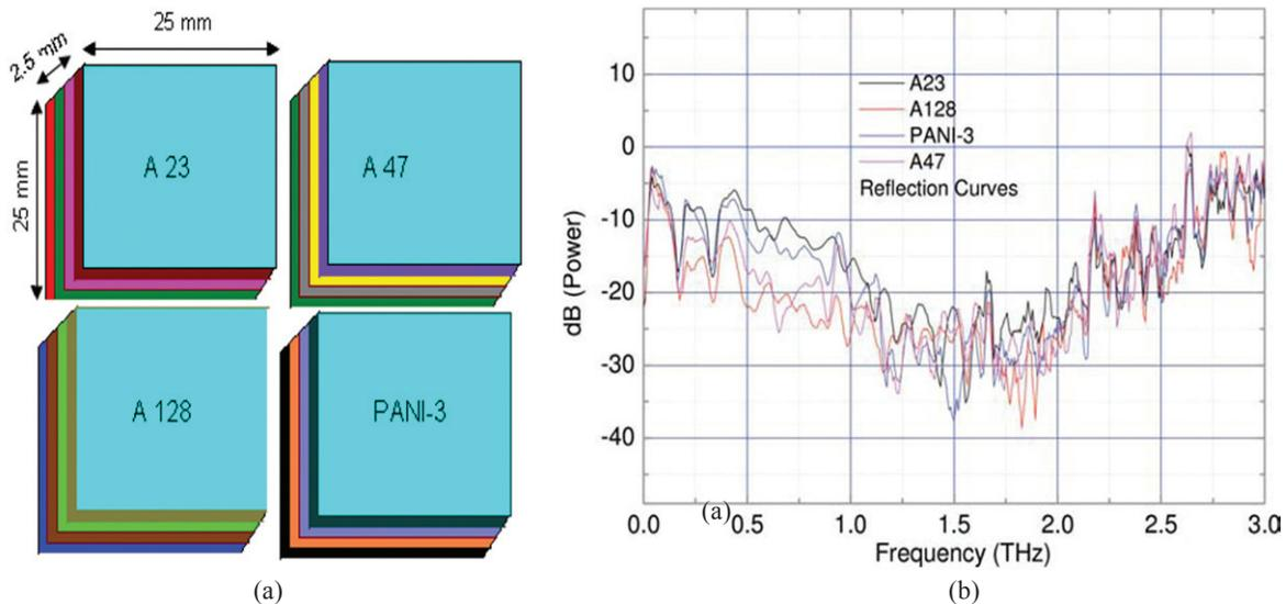
Figure 9. Schematic of fabricated structures (a) reflection loss measurements and (b) polymeric coating in THz region<sup>16</sup>.
