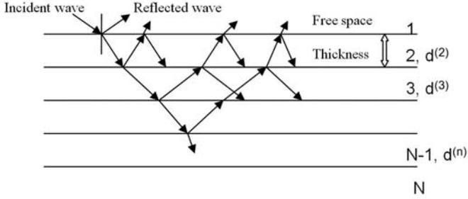
**Figure 2. Multilayer absorbing structure backed by a perfectly conducting plate.**
