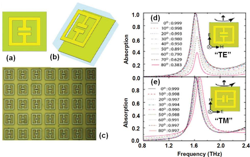
Figure 8. Flexible wide angle THz absorber and numerical calculations for high absorption over a wide range of angles of incidence for both TE and TM radiation<sup>14</sup>.
