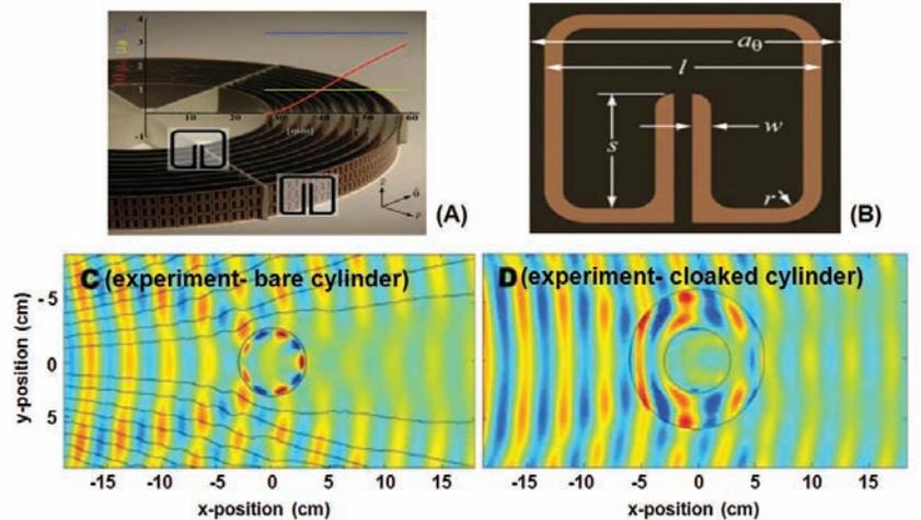
**Figure 3. First experimental demonstration of cloaking at 8.5 GHz<sup>8</sup>.**
