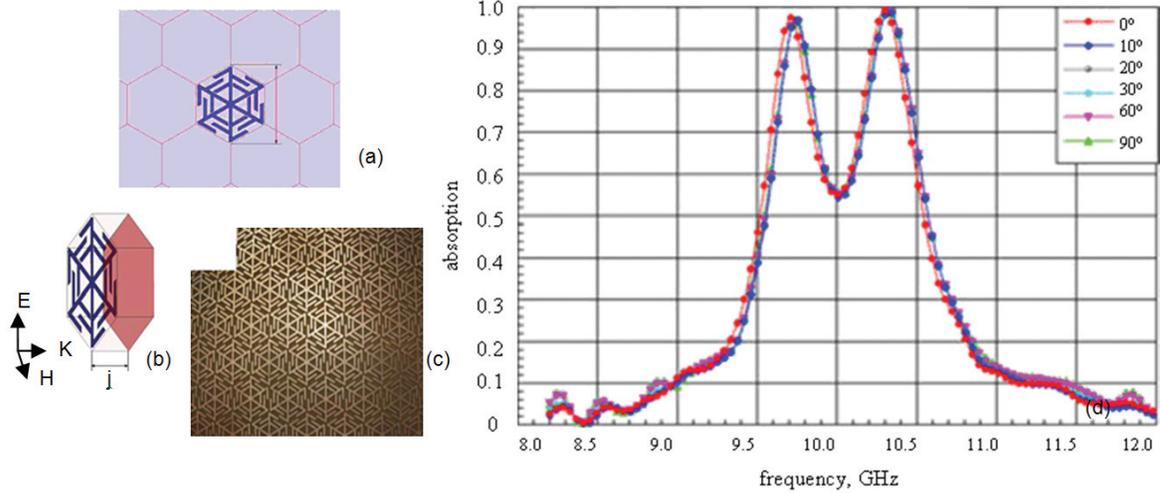
Figure 5. Bandwidth enhanced double resonance metamaterial absorber<sup>11</sup>.
