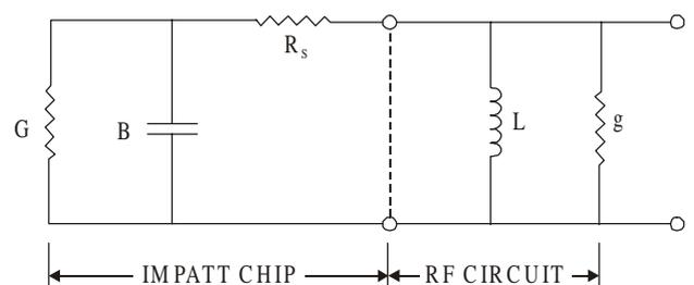
Figure 1. Equivalent model of IMPATT diode without package.
