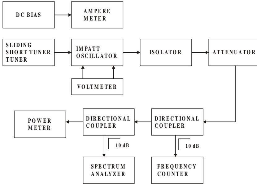
Figure 5. Block diagram of Ka-band measurement test setup.
