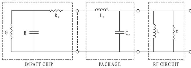
Figure 2. Equivalent model of IMPATT diode with package.
