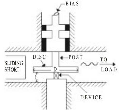
Figure 4. Schematic diagram of Ka-Band resonant cap cavity.
