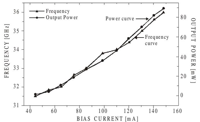
Figure 7. Dc bias current vs frequency and output power.
