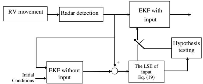
Figure 2. The mechanism of the proposed filter scheme.
