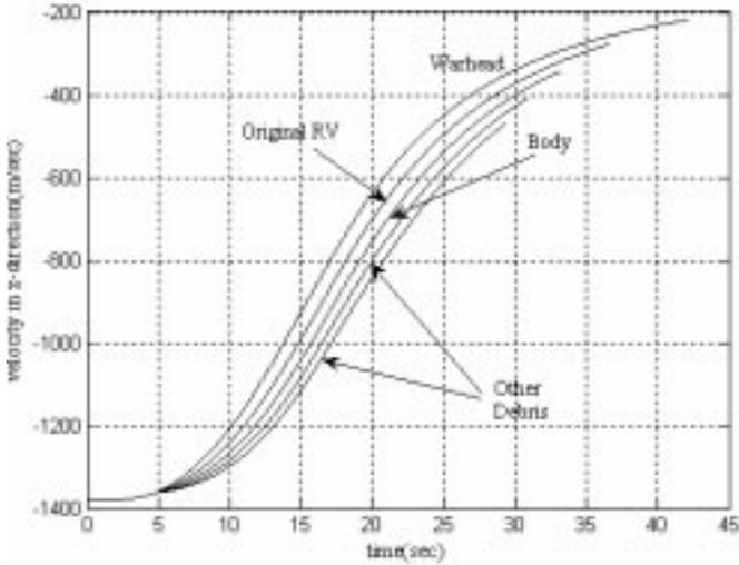
Figure 9. The measured velocity of objects in  $Z_R$ .
