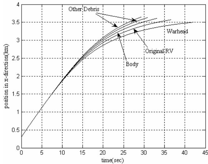
Figure 4. The measured position of objects in downrange.
