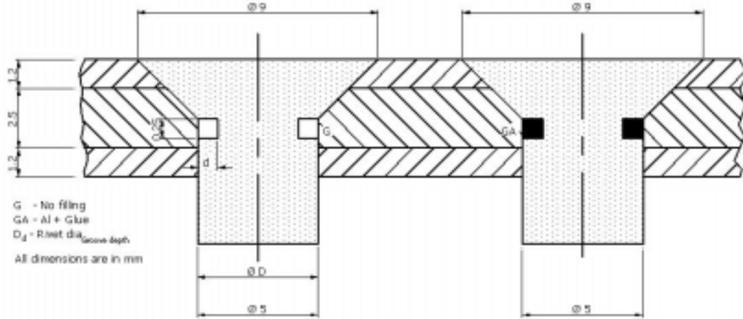
Figure 4. Nomenclature of artificial grooves in the countersunk regions of rivets in panel S7 filled with simulated corrosion product.
