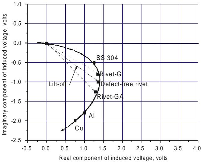
Figure 7. Universal impedance plane diagram for reflection type ring EC probe showing the lift-off response for different electrically conducting materials.
