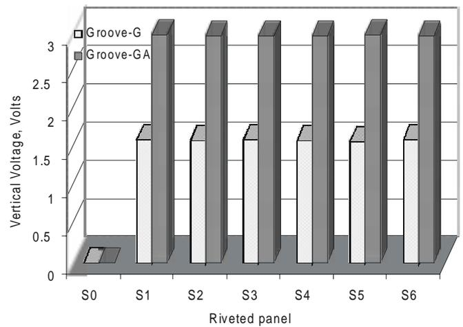
Figure 10. Detection performance of the EC procedure for  $4_{0.5}$  riveted panels with various combinations of multi-layers at optimum test conditions.
