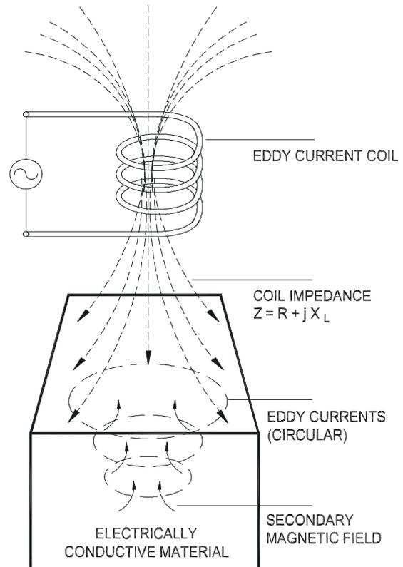
**Figure 2. Principle of eddy current testing.**
