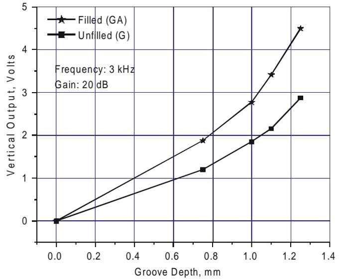
Figure 9. EC response for 5 mm diameter rivets with unfilled and filled grooves.
