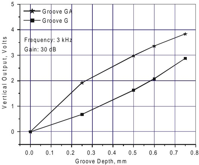
Figure 8. EC response for 4 mm diameter rivets with unfilled and filled grooves.
