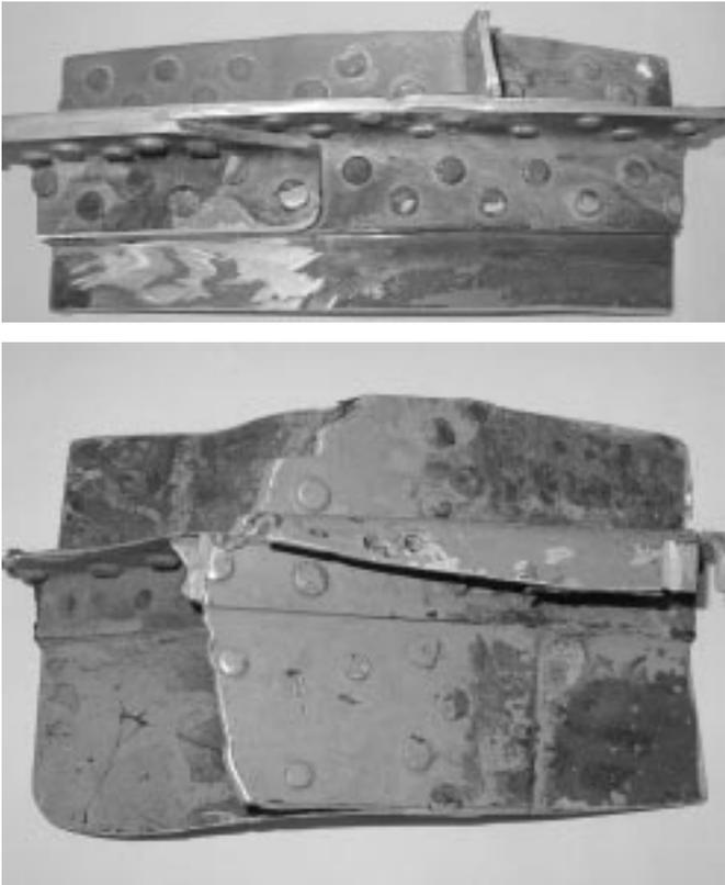
**Figure 1. Photographs of a portion of riveted panels from a failed aircraft (Cat-E).**
