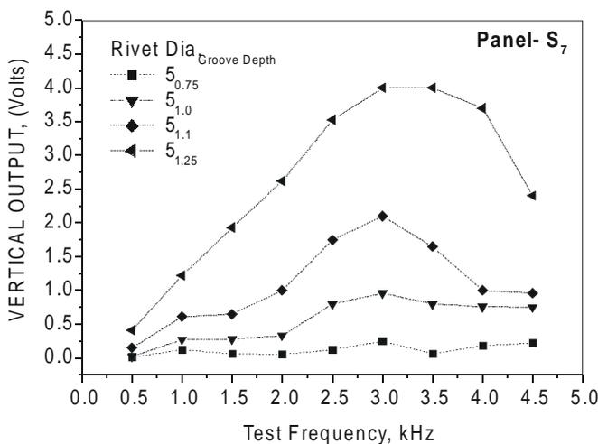
Figure 5. Optimisation of test frequency. At 3 kHz (depth of penetration of eddy currents ~ 2 mm), EC response from grooves shows a distinct peak.
