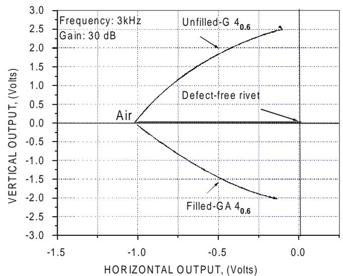
Figure 6. Typical EC signals from 4 mm dia. defect-free rivet and rivets with filled (GA) and unfilled (G) grooves.
