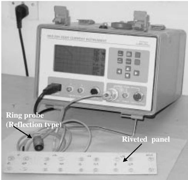
**Figure 3. Reflection type ring probe connected to EC instrument for detection of defects in countersunk regions of rivets.**
