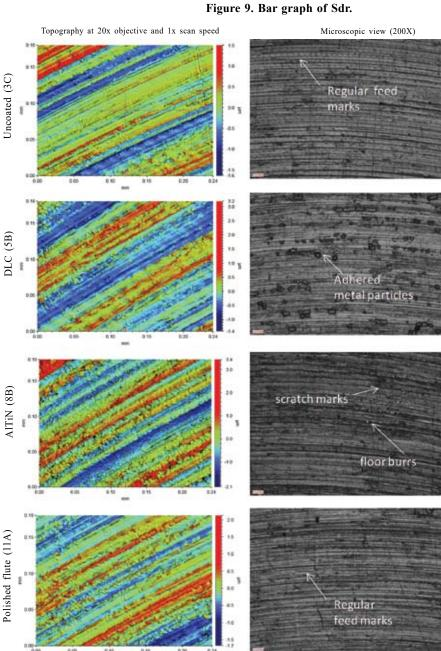
Figure 10. Topographic images of the aluminium alloy surface machined at 10  $\mu$ m/ tooth and depth of cut 0.25 mm with various coatings and processed solid carbide tools.
