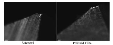
Figure 4. Uncoated and polished cutting tools edge after machining at 500X.
