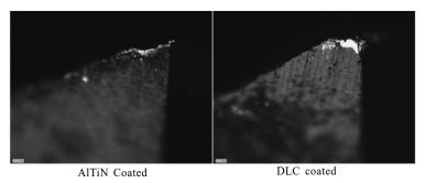
Figure 5. AlTiN and DLC coated cutting tools edge after machining at 500X.
