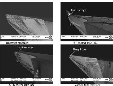
Figure 6. SEM images of cutting tools rake face after machining at 700X.
