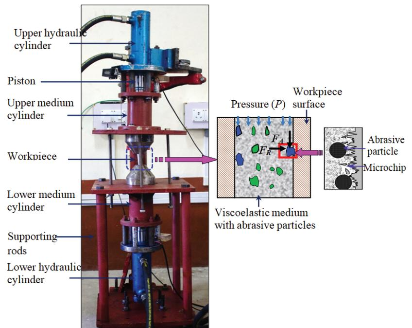
Figure 1. Abrasive flow finishing process set-up with various finishing forces on abrasive particle during the process.
