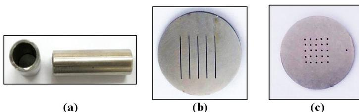
Figure 3. Various workpieces finished by the abrasive flow finishing process (a) tubes having inner diameter 12.7 mm, (b) microslots having length 20 mm and width  $450\ \mu\text{m}$ , and (c) microhole having radius  $425\ \mu\text{m}$ .
