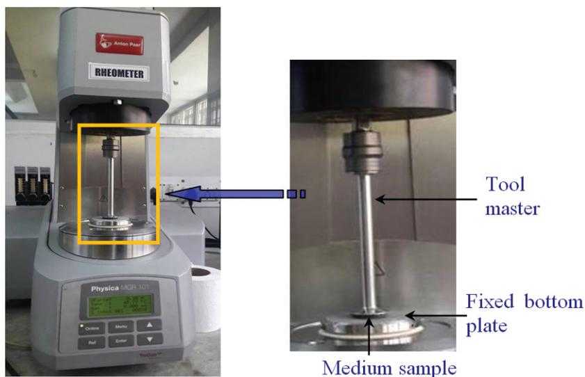
Figure 2. Parallel plate rheometer with sample between top and bottom plate.
