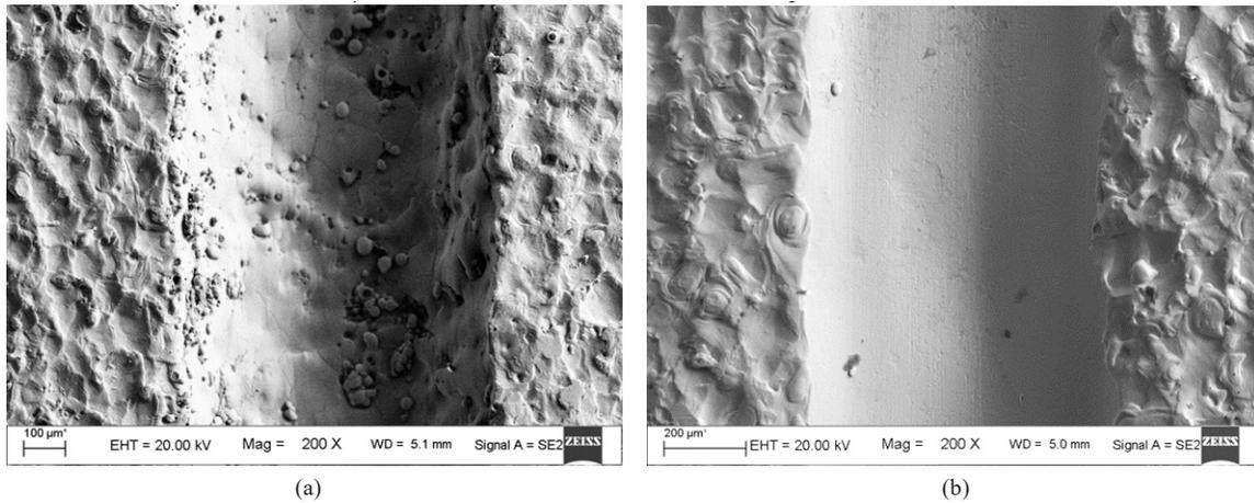
Figure 7. Topography of the microhole surface (a)  $R_a = 1.43 \mu\text{m}$ , initial and (b)  $R_a = 0.17 \mu\text{m}$ , after abrasive flow finishing (wt. % of abrasive particle = 45 %).
