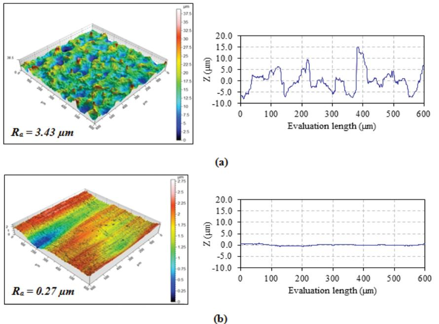
Figure 6. Topography of the microslot surface (a) initial (b) after abrasive flow finishing (wt. % of abrasive particle = 45 %).
