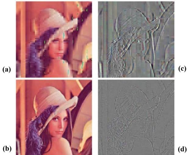
**Figure 4.** Image generated by dropping the errors and just using the straight line parameters. Hilbert image (b) retains better clarity when compared to the normal image (a). The corresponding errors when viewed as images. The errors of the normal image (c) reveals more about the image than its Hilbert counterpart (d).
