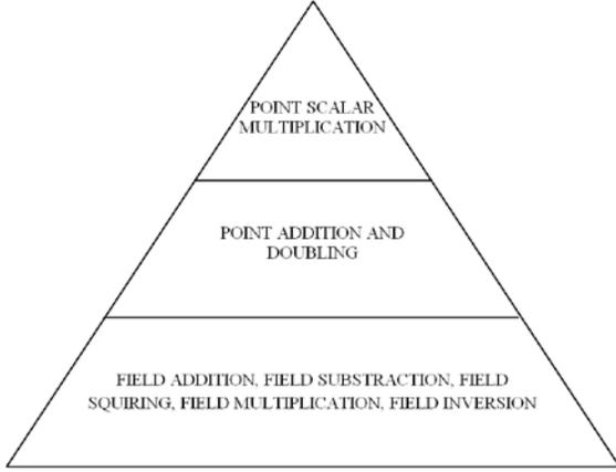
**Figure 2. The hierarchy of operations in the elliptic curve point scalar multiplication operation.**
