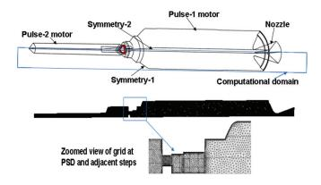
Figure 3. Computational geometry along with grid in the plane of symmetry 2.
