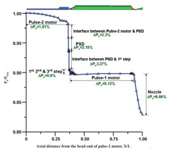
Figure 10. Area averaged total pressure distribution in the axial direction.
