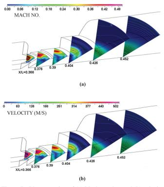
Figure 7. Blown up view of (a) Mach number and (b) velocity distribution in PSD and adjacent pulse-1 motor.
