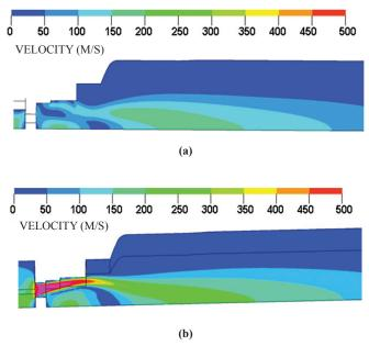
Figure 8. Velocity distribution in (a) symmetry-1 (b) symmetry-2 at PSD and pulse 1 motor
