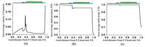
Figure 9. Axial distribution of area average (a) Axial velocity, (b) Static pressure, and (c) Static temperature.
