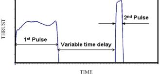
Figure 2. Typical thrust-time history of a dual pulse rocket motor.
