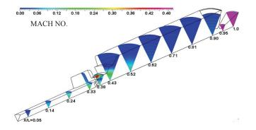
Figure 6. Mach number distribution at various axial locations in the rocket motor.
