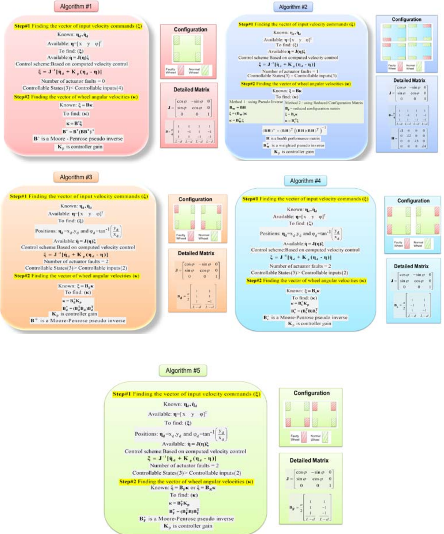
Figure S4. Algorithmic representation of the proposed fault tolerant control scheme.
