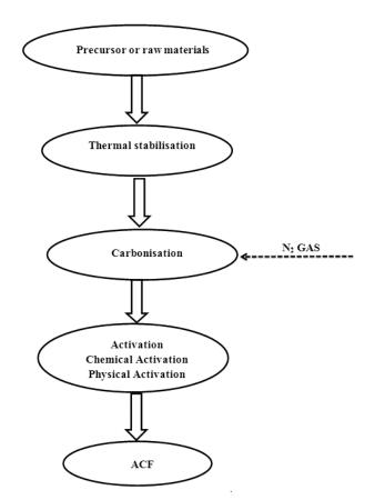
Figure 1. Process flow diagram for preparation of ACF.
