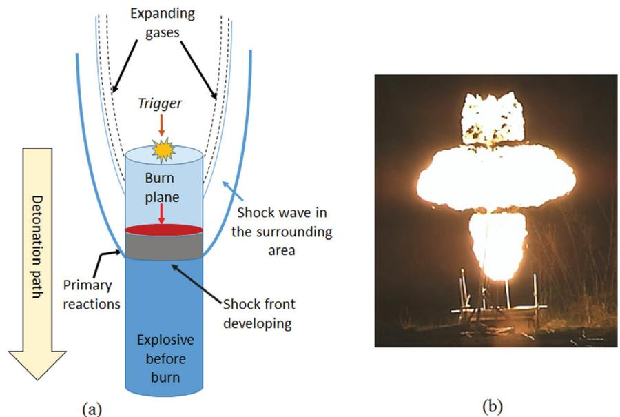
Figure 1. (a) Typical pattern of development of cylindrical shape explosive detonation. (b) Detonation of a cylindrical shape explosive triggered on top. Image 1.6 ms after trigger.
