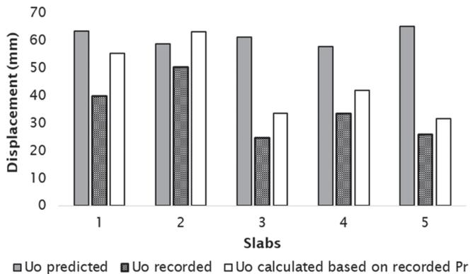
Figure 6. Comparison of predicted and recorded maximum displacement with predicted values.
