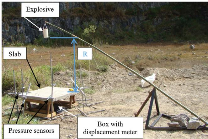
**Figure 3. Test setup.**
