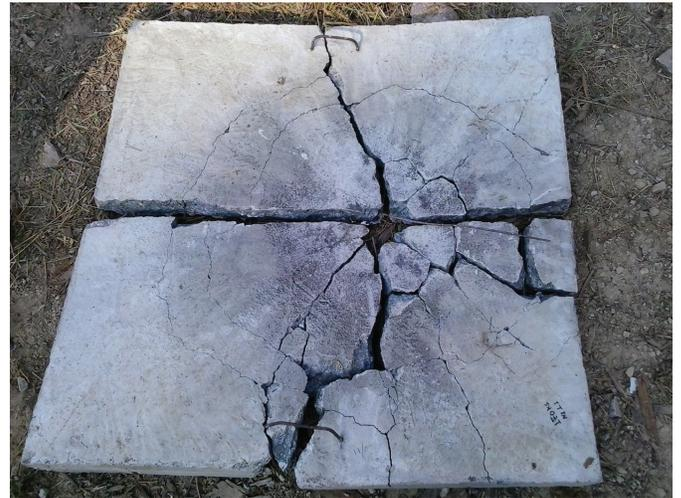
**Figure 4. Slab A post-test. Circular cracks were developed on the upper surface.**
