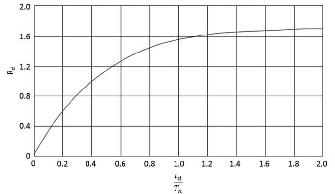
Figure 2. Shock spectra for triangular pulse.
