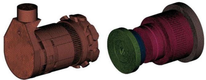
**Figure 5. Optimised geometry (stationary fluid mesh, rotating fluid mesh, solid mesh - Stator rotor windings and core mesh and yoke).**
