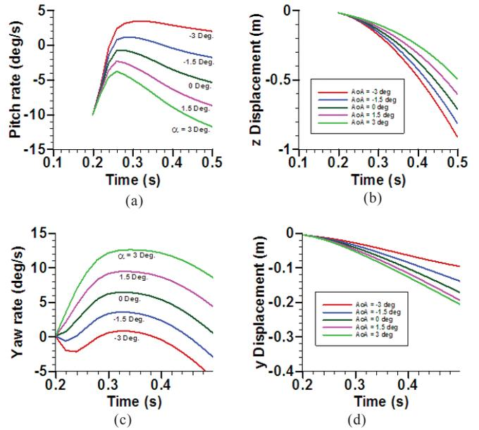
Figure 5. Effect of angle of attack of aircraft on missile trajectory; (a) pitch rate, (b) vertical displacement, (c) yaw rate, and (d) lateral displacement.
