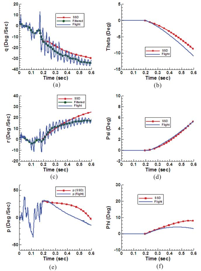
Figure 8. Comparison of body rates and angles with the flight data; (a) pitch rate, (b) pitch angle, (c) yaw rate, (d) yaw angle, (e) roll rate, and (f) roll angle.
