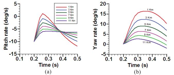
Figure 6. Effect of launch altitude on missile trajectory; (a) pitch rate and (b) yaw rate.
