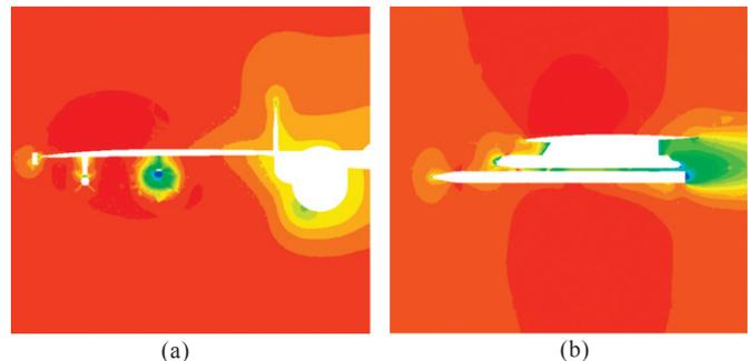
Figure 3. Mach contours in a : (a) cross-section and (b) pitch plane.
