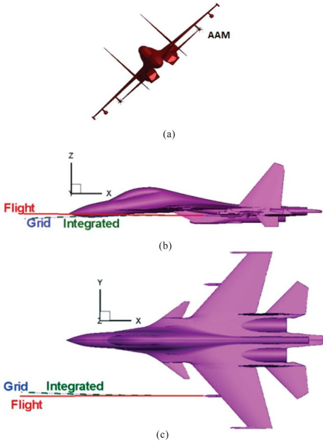
Figure 7. Comparison of predicted displacement of missile with the flight data; (a) Level turn Manoeuvre, (b) Relative displacement (side view), and (c) Relative displacement (Top view).
