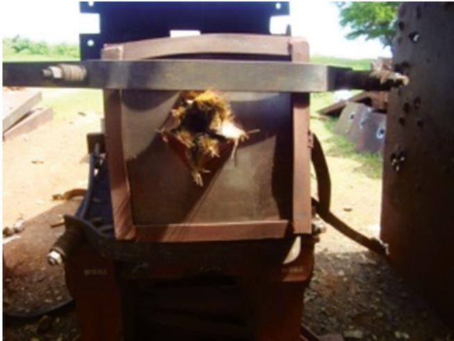
**Figure 8. DOP test configuration.**
