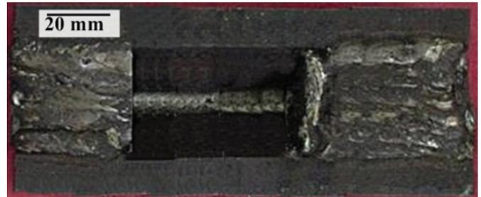
**Figure 1. 80 mm Tekken specimen after welding.**
