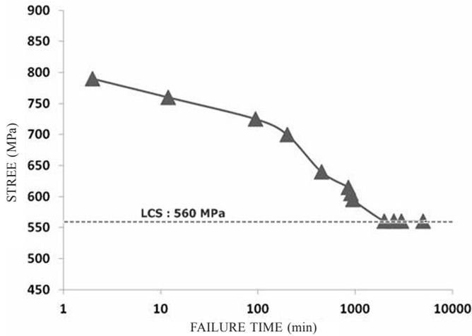
Figure 3. Stress-time curve for 500 °C tempering condition.
