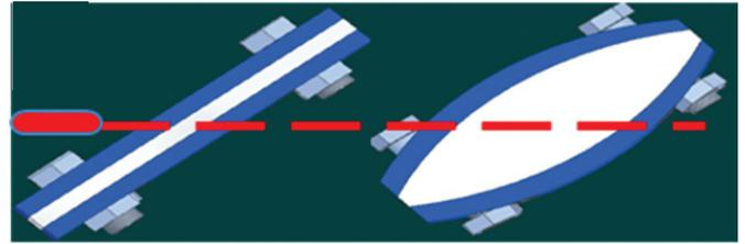
Figure 10. Working principles of non explosive reactive armour.
