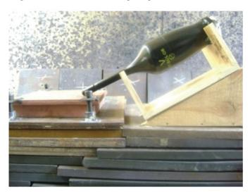
Figure 9. Experimental set up for ballistic evaluation of ERA against shaped charge warhead.
