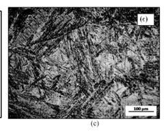
Figure 2. Microstructure of 500 °C tempered 80 mm thick Tekken specimens (a) Base metal, (b) Base metal – weldments interface, and (c) HAZ.
