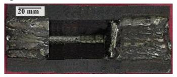
Figure 1. 80 mm Tekken specimen after welding.
