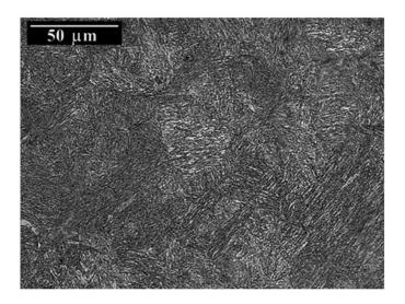
Figure 6. Optical microstructure of 50 mm DMR 1700 steel plate.
