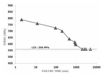
Figure 3. Stress-time curve for 500 °C tempering condition.
