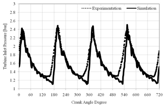
Figure 11. Turbine inlet pressure pulsations comparison.
