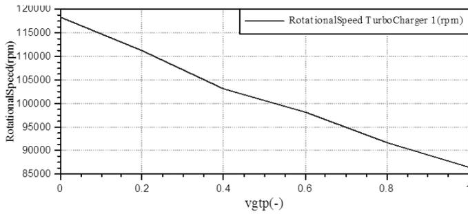
Figure 13. Effect on rotational speed of VGT.
