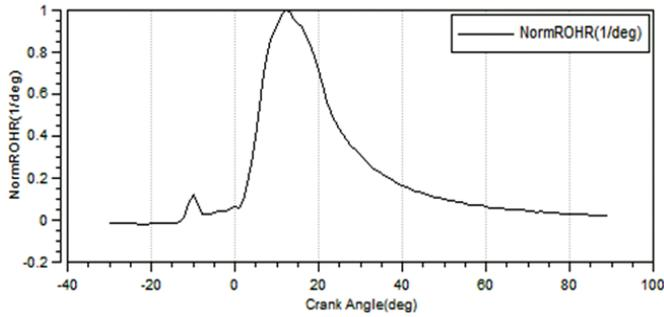
Figure 4. Combustion data as rate of heat release.
