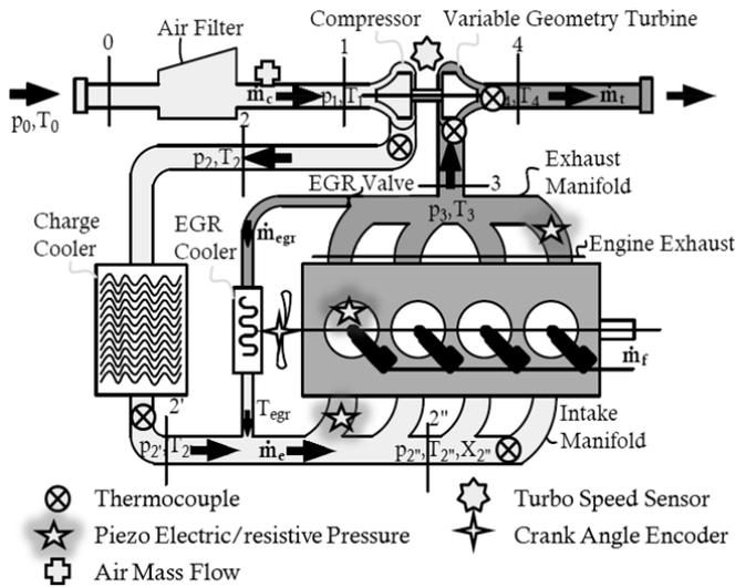
Figure 8. Instrumentation layout.
