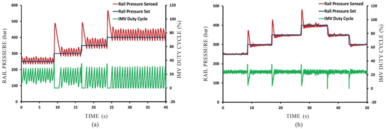
Figure 8. Fuel rail pressure controller tuning - response of a poorly tuned controller with  $K_p=0.5$ ;  $K_i=0$ ;  $K_d=0$  as shown in (a) vs a well tuned controller with  $K_p=0.2$ ;  $K_i=0.05$ ;  $K_d=0$  as shown in (b).
