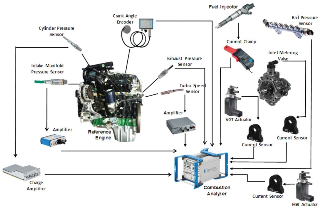
**Figure 1. High speed data acquisition layout<sup>5</sup>.**
