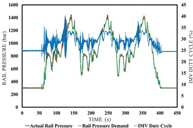
Figure 12. Performance of the rail pressure controller during transient cycle.
