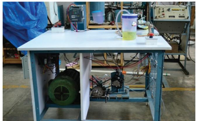
Figure 7. In-house developed fuel injection test rig.
