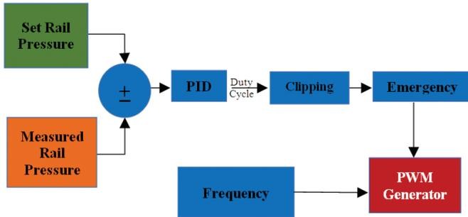
Figure 5. Fuel rail pressure control algorithm.
