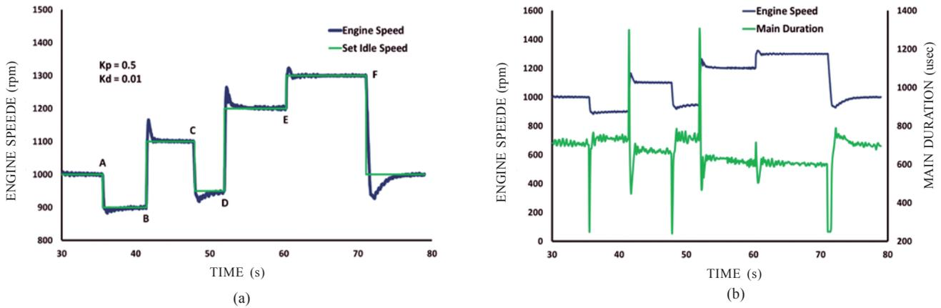
Figure 9. (a) Response of idle speed controller to changes in set idle speed and (b) Controller action taken against changes in set idle speed.
