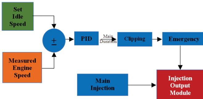
Figure 6. Low-Idle speed control algorithm.
