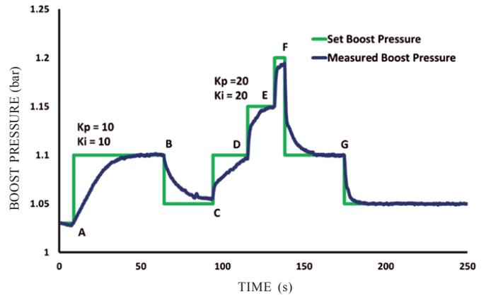
Figure 10. Typical boost controller calibration activity.
