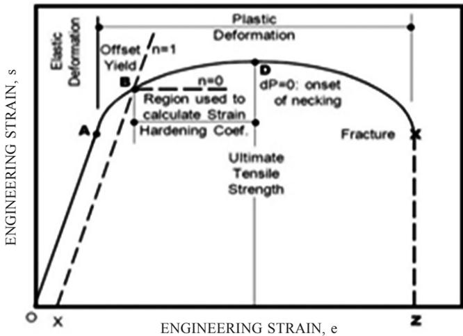
Figure 5. Material curve.
