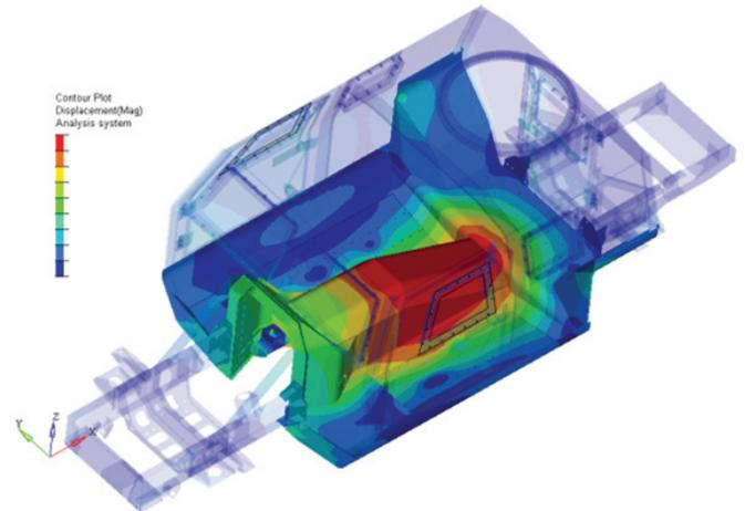
Figure 7. Local deformation of the vehicle.
