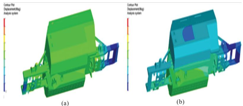
Figure 8. (a) Loading at centre hull and (b) Loading at driver side.
