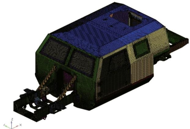
Figure 3. Armoured vehicle: Finite element model.
