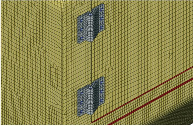
Figure 4. Hinges and weld elements.
