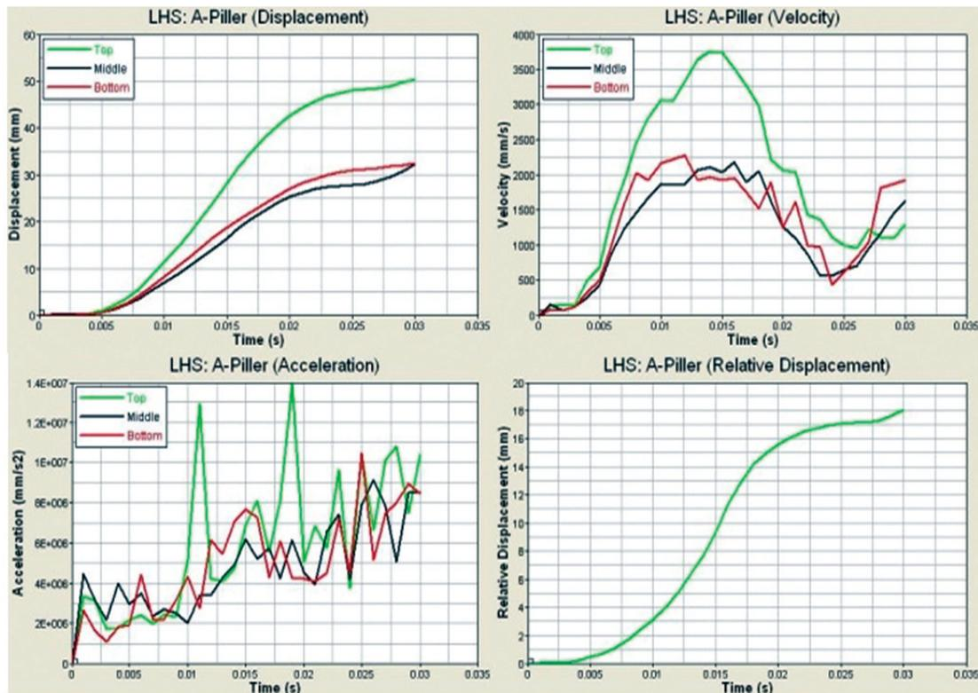
Figure 11. Displacement, velocity, acceleration plots.
