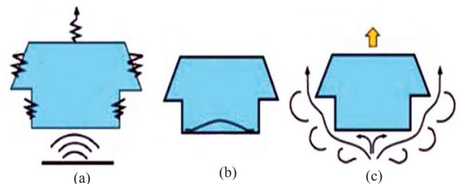
Figure 1. Blast process phases: (a) Blast wave, (b) local deformation at the bottom of the vehicle, and (c) global displacement of the vehicle.
