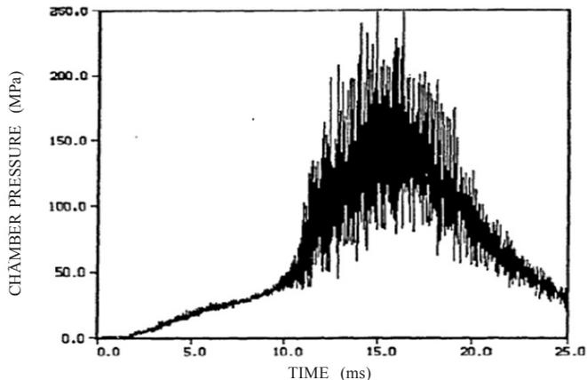
Figure 6. Pressure-time history Crusader gun system<sup>6</sup>.
