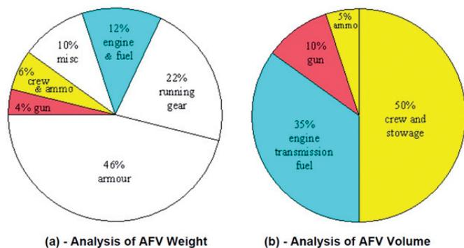
**Figure 10. Effect of armour on weight and volume<sup>9</sup>.**
