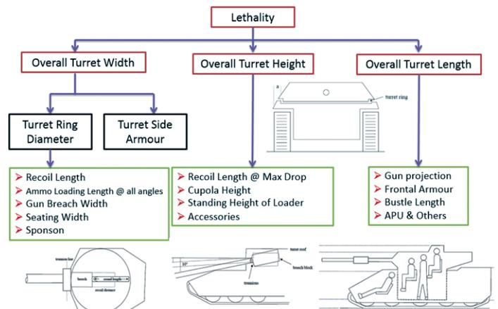
Figure 4. Effect of armament system on configuration<sup>3</sup>.
