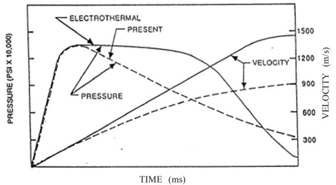
Figure 8. Pressure and velocity-time history for general dynamics gun system<sup>7</sup>.
