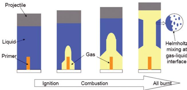
Figure 5. Ignition cycle for bulk loaded LPG system<sup>4</sup>.
