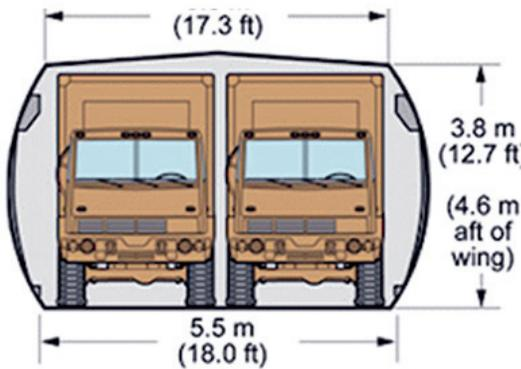
Figure 15. C-17 globemaster ODC profile<sup>16</sup>.
