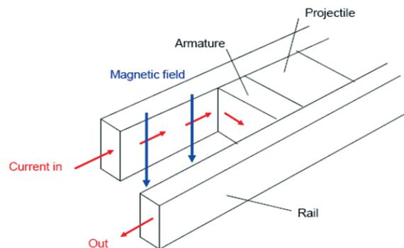
Figure 9. Typical EM Gun system working principle.
