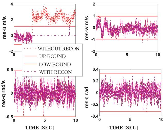
Figure 9. Residuals with/without reconfiguration using fuzzy logic for fault in 1st channel.
