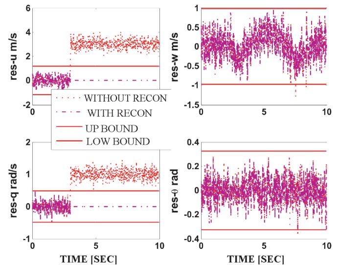
Figure 11. Residuals with/without reconfiguration using fuzzy logic for faults in 1<sup>st</sup> and 3<sup>rd</sup> channels.
