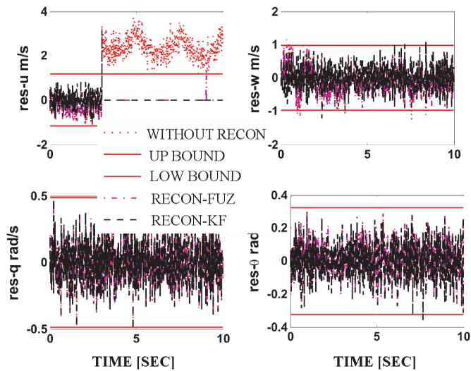
Figure 12. Residuals with/without reconfiguration using fuzzy logic and KF for faults in 1<sup>st</sup> channel.
