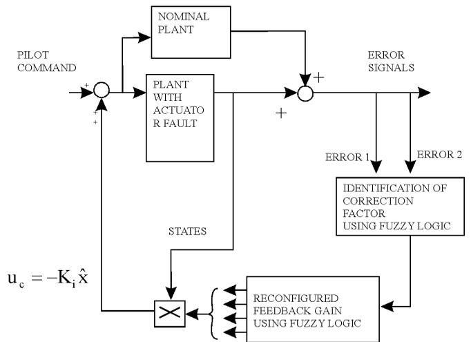
Figure 5. System identification and reconfiguration using state feedback.
