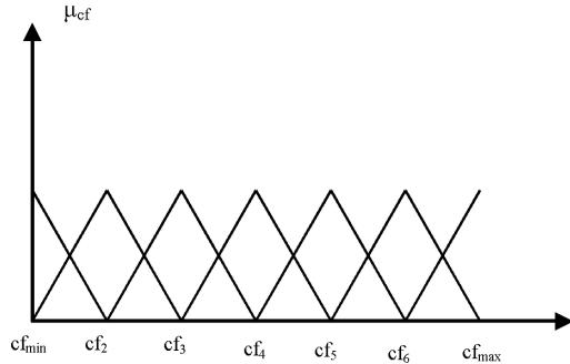
Figure 7. Membership functions for output correction factor (cf).
