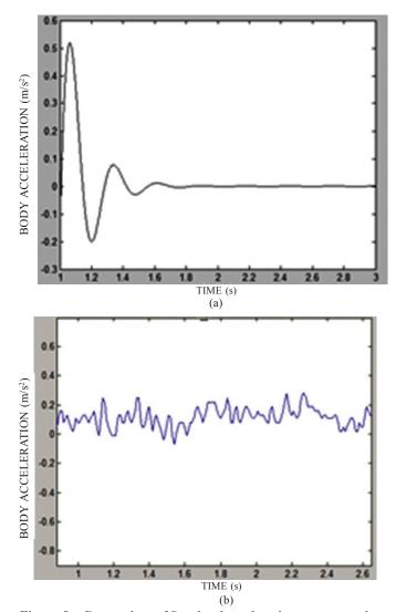
Figure 8. Comparison of Seat level acceleration response values obtained through modelling and simulation study with the case study results (a) Acceleration (m/s<sup>2</sup>) at seat level (obtained through modeling and simulation) for old parameter values (b) Acceleration (m/s<sup>2</sup>) at seat level (obtained through case study) for old parameter values.
