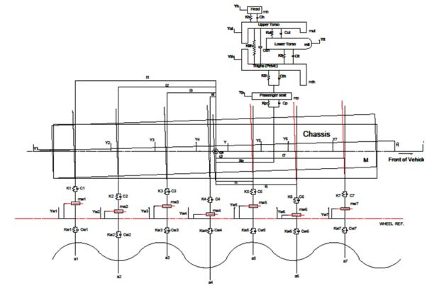
Figure 1. Vehicle-occupant composite model.
