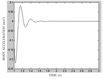
Figure 9. Acceleration (m/s<sup>2</sup>) at seat level (obtained through modelling and simulation) for optimised seat suspension parameter values.
