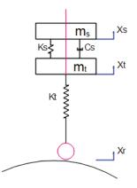
Figure 2. Occupant-seat suspension model.
