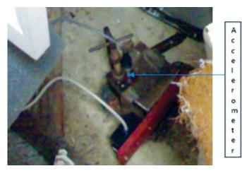
Figure 3. Mounting of accelerometer.
