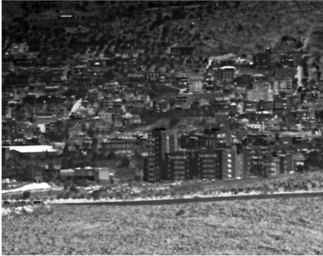
Figure 8. Image registered with the 15 \mu m pitch, 640 \times 512 Pelican-D LW FPA operating with F/2.7 optics at 77K (Scene distance = 5 Km).
