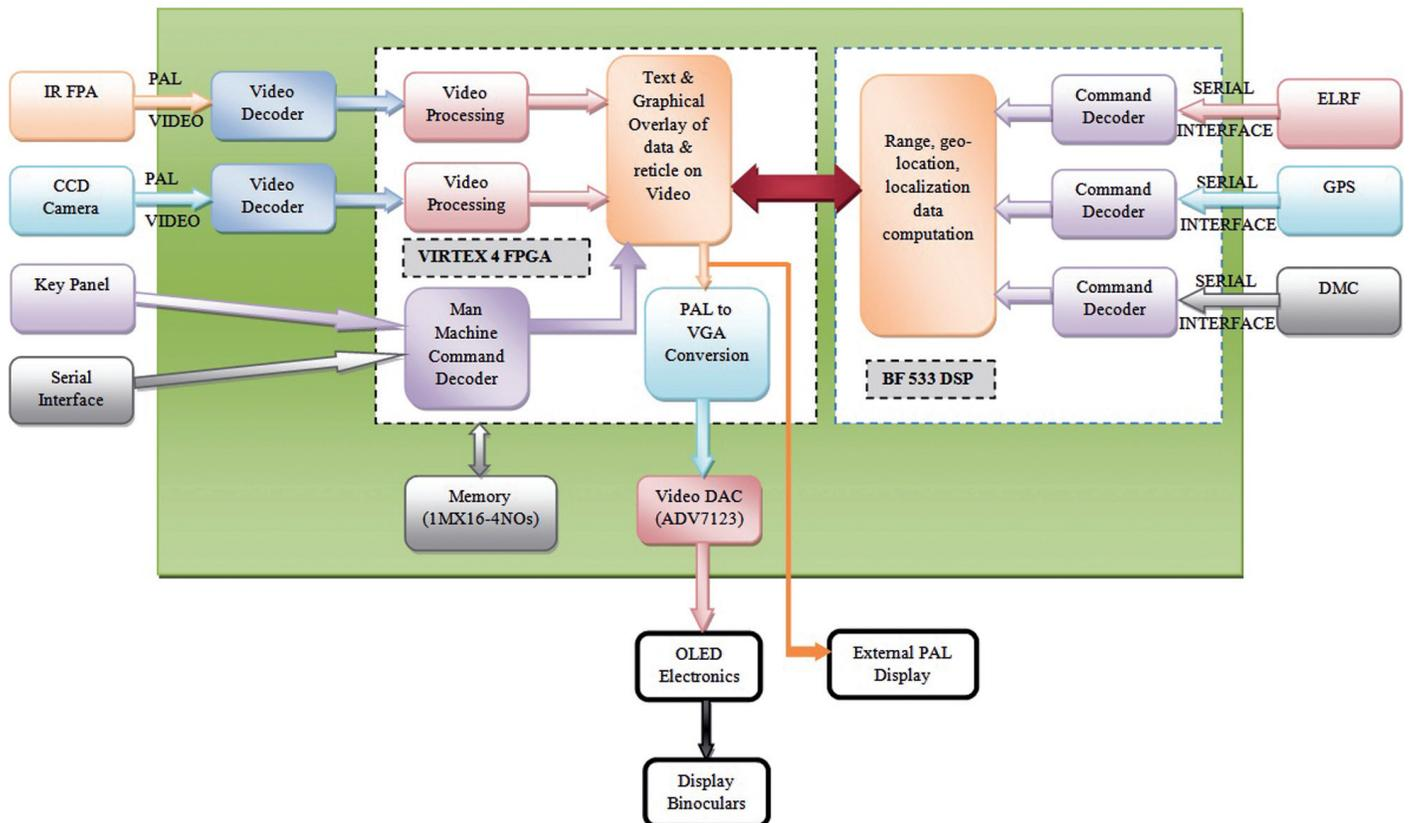
Figure 1. Block diagram of signal processing electronics.
