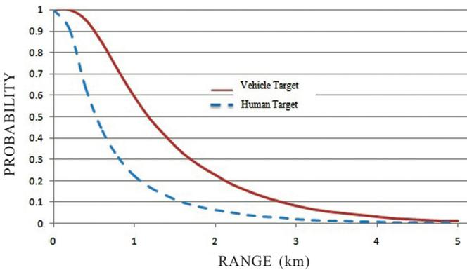
Figure 2. IR imager range simulation results for vehicular and human targets.
