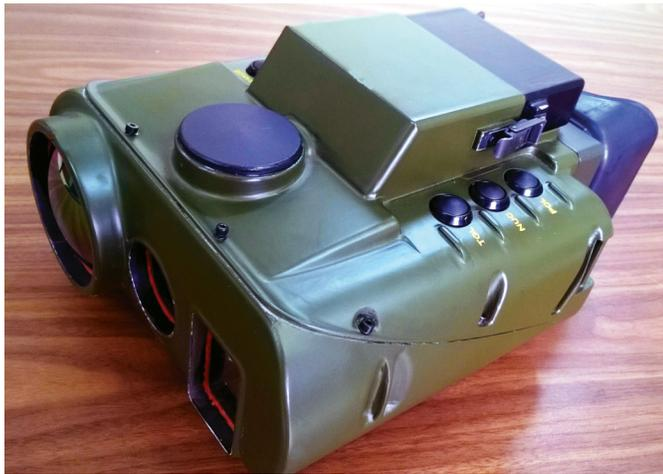
Figure 6. Hand held target acquisition device.
