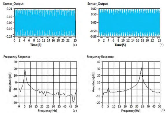
Figure 4. (a) Open-loop responses when the beam is excited at first mode, (b) open-loop responses when the beam is excited at second mode, (c) open-loop frequency responses when the beam is excited at first mode, and (d) Open-loop frequency response when the beam is excited at second mode.
