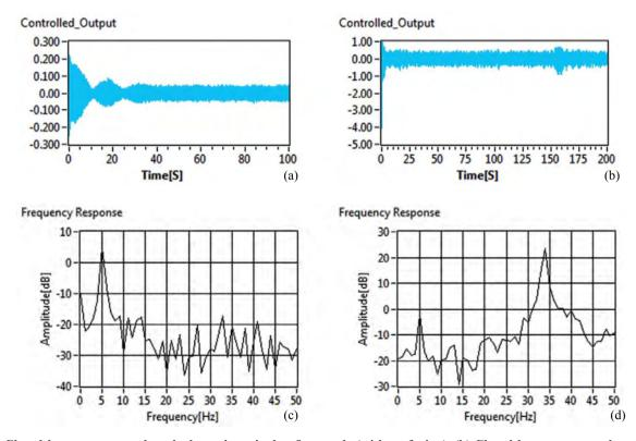
Figure 5. (a) Closed-loop responses when the beam is excited at first mode (without fusion), (b) Closed-loop response when the beam in excited at second mode (without fusion), (c) Closed-loop frequency response when the beam is excited at first mode (without fusion), and (d) Closed-loop frequency responses when the beam in excited at second mode (without fusion).
