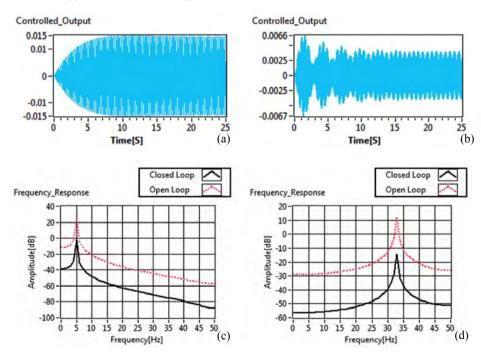
Figure 3. Closed-loop responses when the beam is excited with fusion: (a) at first mode, (b) at second mode; Closed-loop response when the beam is excited with fusion, (c) at first mode, (d) at second mode; open and closed-loop frequency response when the beam in excited with fusion.
