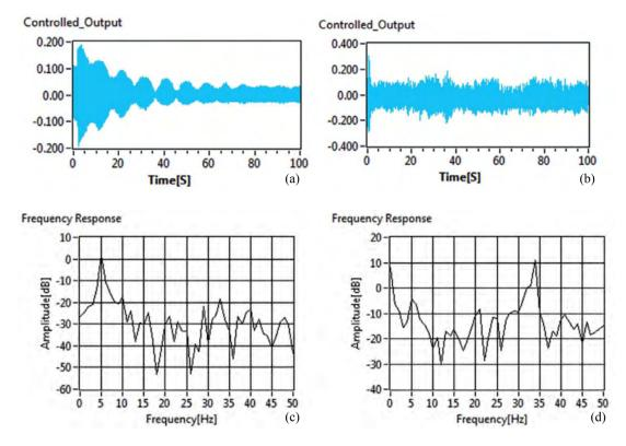
Figure 6. (a) Closed-loop response when the beam in excited at first mode (with fusion), (b) Closed-loop response when the beam in excited at second mode (with fusion), (c) Closed-loop frequency response when the beam in excited at first mode (with fusion), and (d) Closed-loop frequency response when the beam in excited at second mode (with fusion).
