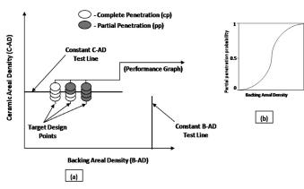
Figure 1. (a) Design of experiments in protective areal density (PAD) test configuration and (b) fitting of binomial ballistic test data.
