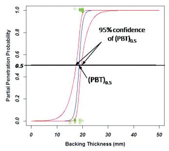
Figure 6. The complete S-shaped binary response curve for protective backing thickness of Al 2024-T351 backing, in a PAD test configuration with strike face of 12.2 mm thickness hot pressed boron carbide tiles confined in steel, against 12.7 mm AP ammunition.
