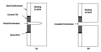
Figure 3. Schematic diagram of the PAD test target configuration (a) Partial Penetration (pp), and (b) Complete Penetration (cp).
