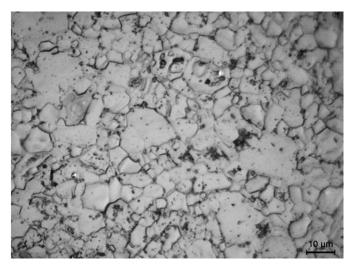
Figure 2. Microstructure of hot pressed boron carbide tile.
